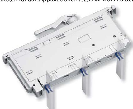
The SASILplus system is versatile. Versions for 2-pole, 3-pole and 4-pole construction are also available as well as for the 185mm and 60mm busbar systems.
